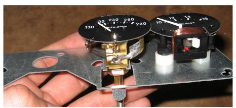
The gauge is properly located when it sits fully into the curved pocket in the mounting tab.
