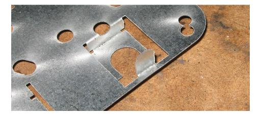
No bends are needed for locations with an electrical gauge (including the voltmeter/ammeter with the mechanical gauge set).
