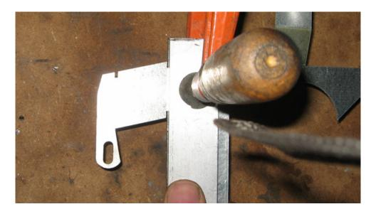
And finally bend the outer tabs down between the outer notch and the corner:
