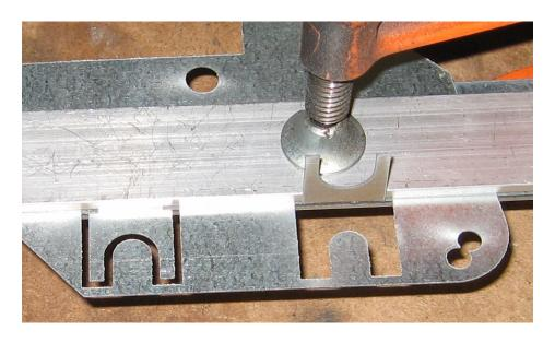
Then bend it back down at the upper notches. This creates a Z-bend that lowers the mounting tab into the gauge cluster:
