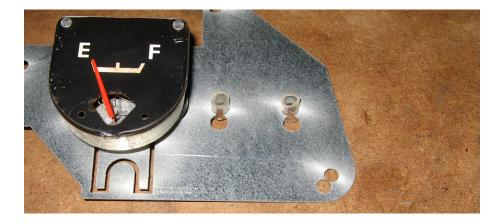
Slip any spacers or washers on the inside of the bracket over the tubing:
