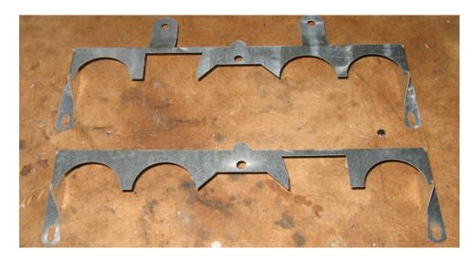
Paint the gauge masks with flat black paint (I like Rustoleum). It is only necessary to paint the outer surface:
