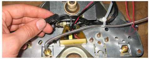
Lastly, install the fuel gauge terminals (for a three-post gauge, only the two outer posts are used), and the ground terminal (attach to any of the bracket screws):
