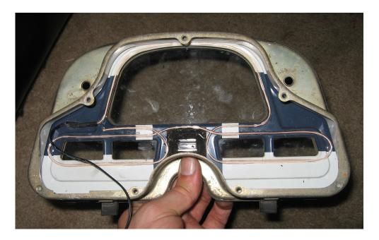
There will be up to 12" of extra wire, simply cut the excess away. You may wish to put a dab of cement on the open end of the wire for waterproofing.
