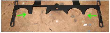
If more correction is needed, you can bend the low edges of the mask, between the gauges, up to create a little standoff. Bend up only about 1/8", do NOT overdo it or you'll end up with gaps by the gauge faces.
