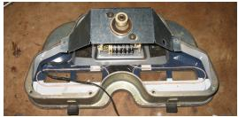
Then set the gauge mask in place as well. Be careful to ensure that you slip the tab in the center of the gauge mask to rest behind (towards the back side of the cluster) the speedometer.
