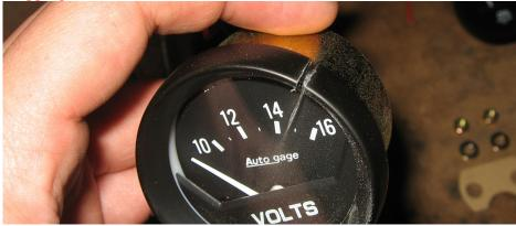
Remove the bezel by simply popping it off and extract the gauge contents. Save the fasteners and the "guts", everything else can be discarded.
