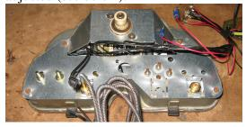
Install the gauges and bracket with five screws. **Don't forget the screw in the center!** Leave all the screws VERY loose until adjustment (see below):
